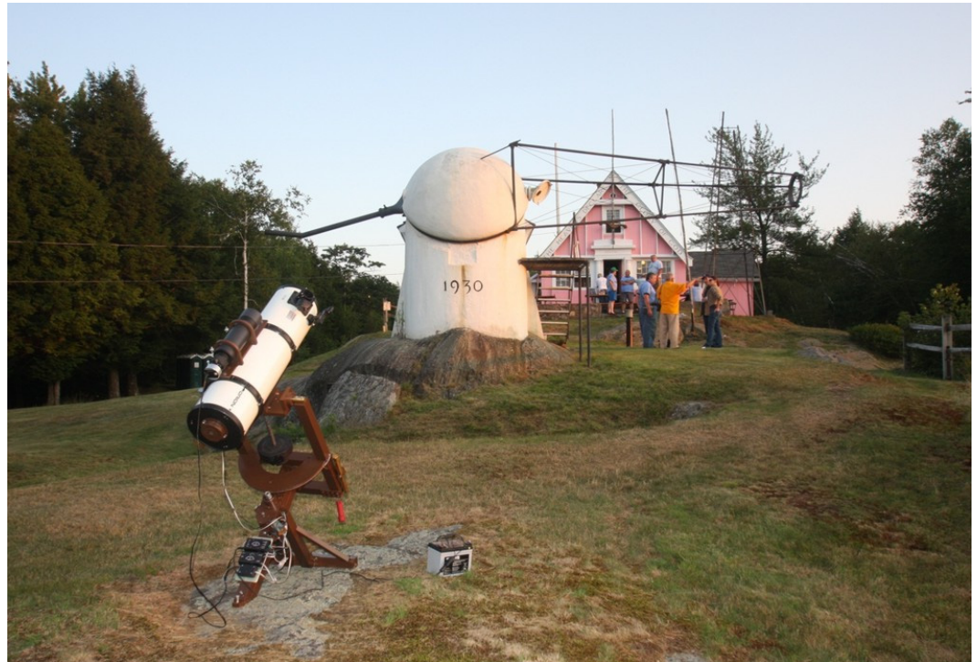
Scott's 7.5 inch Mak/Newt telescope on his full GOTO homemade mount set up next to the famous Porter Turret Telescope at Stellafane, home of the Springfield Telescope Makers.
